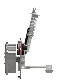
Wheel hub motors and near-wheel drives have not yet become established in the automotive sector. The reasons for this range from increased tire-sprung masses, which lead to a loss of comfort, to increased production costs.
