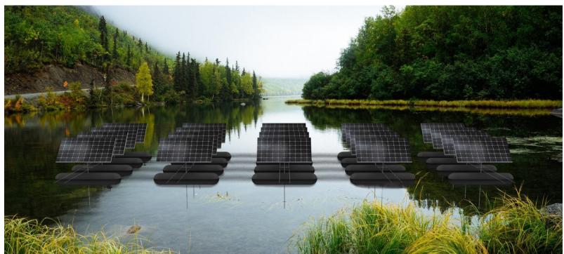
Water surfaces lend themselves to the use of photovoltaics due to their mostly unshaded location. Photovoltaic modules installed on water have a higher energy yield than comparable modules on land due to the reflection of the water and the solar radiation. At the same time, the water has a cooling effect, which also increases output.
